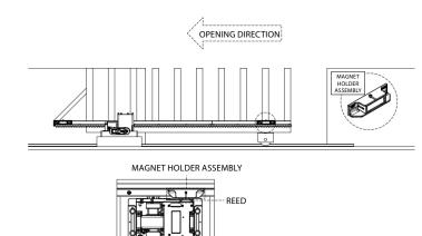
**Step 3:** Run the motor and check if the reeds are correctly turning off. If necessary, reverse the connector of the control board.
