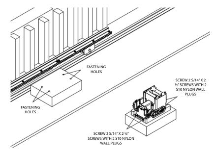
**Step 6:** With the operator manually released, place the rack bar on the pinion, aligned to the gate.
