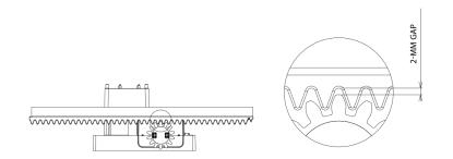
**Step 7:** Fasten the rack bar all along the gate leaf by welding it or by tightening screws every 300 or 400 mm (~ 11.82 or 15.75 in).
