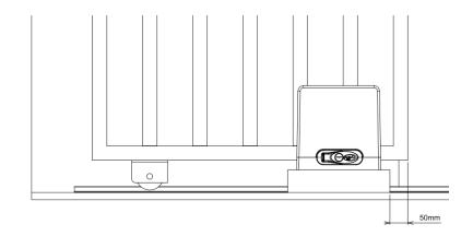
**Step 4:** Perform the pre-alignment of the operator with the gate, by placing the toothed rack on the pinion and leaning this set to the gate. Then, mark the position of the fastening holes on the ground or concrete foundation.
