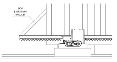
**Step 9:** After fastening the rack bar, fasten the operator permanently to the ground or concrete foundation, by strongly tightening the screws.
