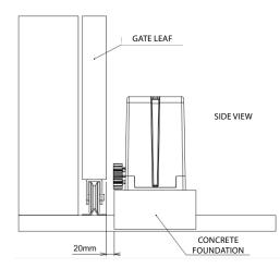
**Step 3:** Once the requirements are complied with, totally open the gate and place the operator near the gate-leaf face, respecting the 50-mm gap between the extremity of the leaf and the concrete foundation.
