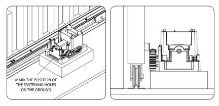
**Step 5:** Drill the fastening holes, by placing the operator level with the gate. Before tightening the S  $\frac{1}{4}$  x 2  $\frac{1}{2}$  screws, move the gate, checking if it does not lean on the operator along its course. If so, move the operator back.
